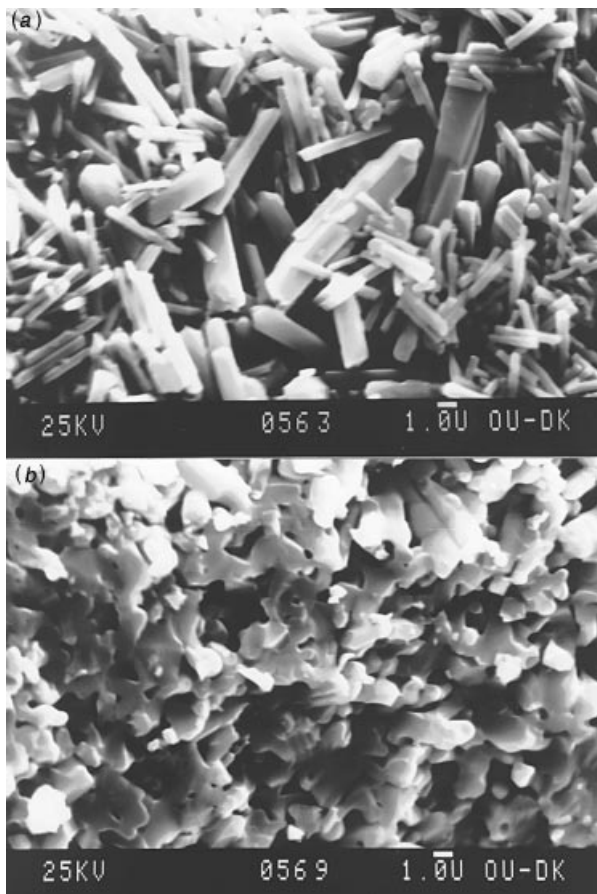
Fig. 5 Scanning electron microscopy photographs of \alpha -LiZnAsO 4 , (a) as synthesised (top) and (b) after two DSC experiments, heating to 900 °C. Magnification, \times 4000 .
